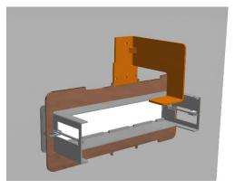
2. Secure the KRT-4-M-V to the underside of the table with two screws.
